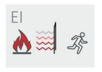
Limits the flow of flames, gases and heat 🕜
